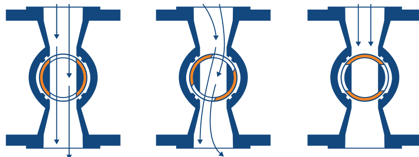
From Left to Right: Full Flow (Plug 0°), Control Flow (Plug Throttling), Shutoff (Plug 90°)
