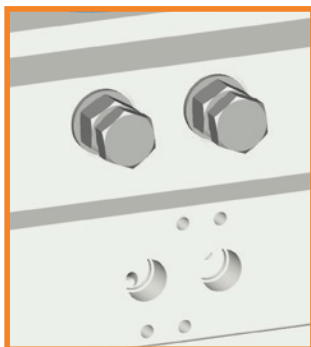
Open/Closed Position Travel Stop Adjustment
